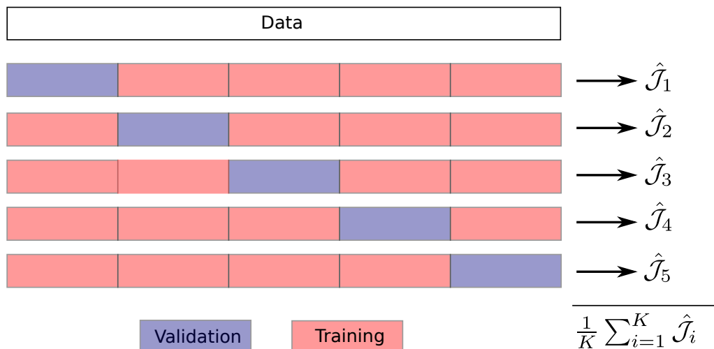
Figure 4.8: Sketch of K -fold cross-validation for K = 5 .
